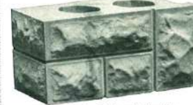
Design No. 4, Broken Ashlar Face. Block made with groove between block sections for bedding or tuck pointing when wall is completed. For fractional blocks order desired division in Design No. 2 which matches this design perfectly. For left hand corner block use Design No. 2 end door. For right hand corner special end door is required.
