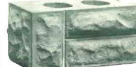
Design No. 3, Broken Ashlar Face. Block made with groove between block sections for bedding or tuck pointing when wall is completed. For fractional blocks order desired division in Design No. 2 which matches this design perfectly. For right hand corner block use Design No. 2 end door. For left hand corner special end door is required.
